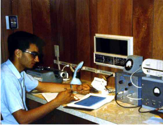
Left: In the age of analog electronics, Tony Mallama is reading the wavering needle of a voltmeter connected to the photometer amplifier. One person in the warm-up room transcribed the meter readings onto paper, while the observer operated the telescope and the photometer in the dome.
